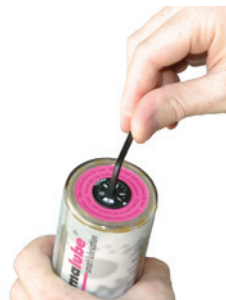
Activate dispensing time with 3 mm Allen key
