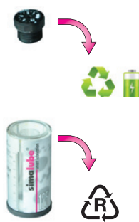
Dispose of intact gas generator in battery recycling and empty housing in plastic recycling. (Warning: dispose of leftover grease separately)
