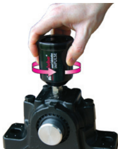
Screw the IMPULSE onto lubrication point
