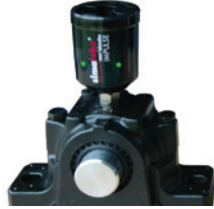
Check and clean the gasket ! IMPULSE remains on lubrication point
