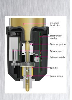
The simalube® IMPULSE ensures reliable lubrication in situations with high counterpressure and long lubrication lines. With the automatic simalube lubricators, this pressure booster pumps greases and oils at up to 10 bar and 0.5 ml per impulse to the targeted lubrication point. The LED display of the intelligent pressure booster provides information continously about the current operating condition, and flashes green when the device is functioning correctly.
