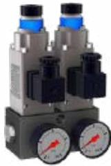
The pressure switch is generally installed upstream of the last lubricant distributor in the main pressure line. It checks the system is working properly.
