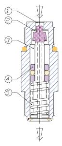
By Operating The Pump, The Pressure Arrives at The Hole (1) And, Through The Tightening of The Valve Lip (2) The Lubricant Enters The Chamber (3) Consequently Moving The Piston (4) Which Supplies The Flow Rate Previously Accumulated In The Chamber (5).
