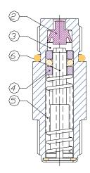
The Piston (4) Has Completed Its Stroke. The Lubricant Has Fully Transferred From Chamber (3) To (5). The Seal Valve (2) Has Closed The Hole (6). The Metering Valve Is Ready For A New Cycle.
