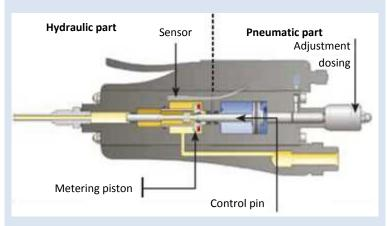
The dosage chamber inlet and outlet are alternatively shut and opened by means of a pin valve with pneumatic control. The dosage chamber volume is continuously adjustable by a lockable screw adjustment.
