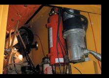
The red Firetrace cylinder can be seen here, along with the red detection tubing as it is run to the critical areas
