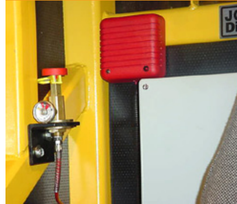
Firetrace offers options such as a manual release option and a warning horn, which is triggered by activation of the system.
