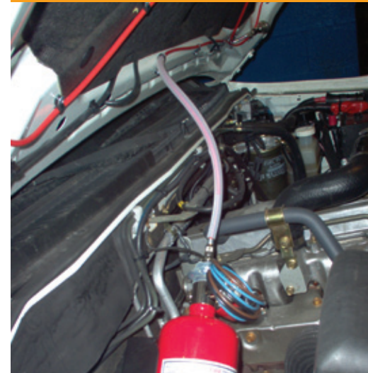
The Firetrace system activates automatically even if the vehicle is unoccupied or has a dead battery.
