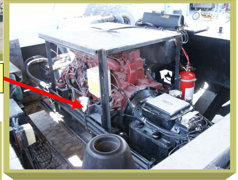
12KG Indirect Powder System Protects main Engine.
