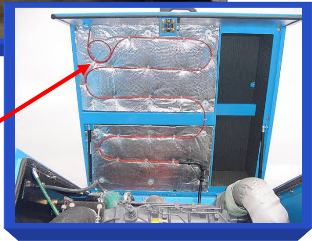
Firetrace Detection Tube installed on inside of insulated engine compartment access flap provides linear heat detection anywhere along its length. Detects fire quickly – wherever it starts!
