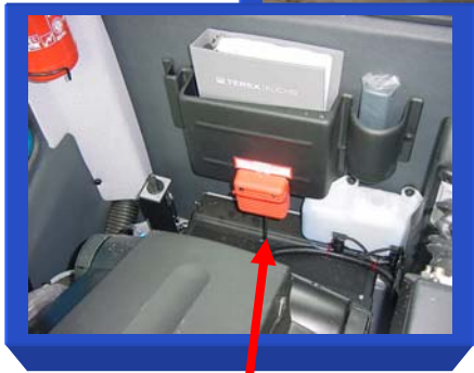
Optional Battery Operated Sounder located in crew cab alerts driver that a fire has been detected.
