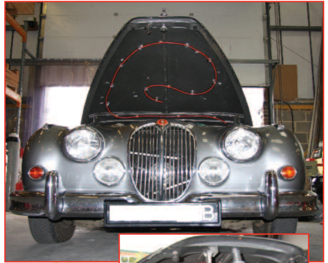
On this project the trace detection tube has been located on the bonnet
