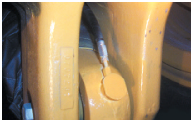
Inlet adaptor designed to protect the compression fitting
