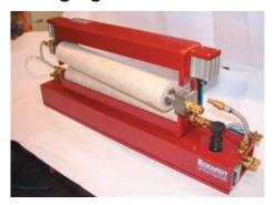
In one basic housing several width of rollers can be mounted (60%rule). You can also mount different rollers for different typs of oil.
