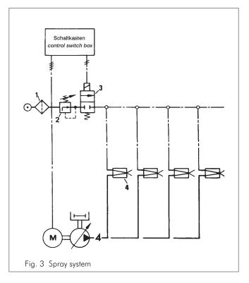
The compressed air necessary for spraying is purified by an air filter (1), regulated by an air regulator (2) and passed to the spray nozzles (4) via a solenoid valve (3).
